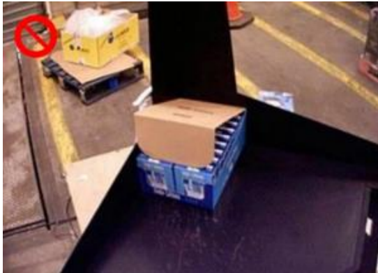
The flap on the top of the case is unsecured/loose
