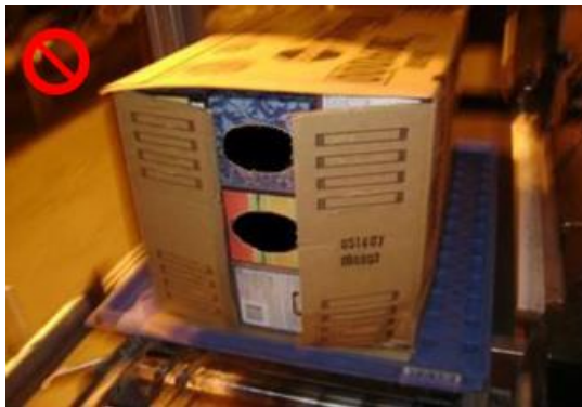
The flap on the side of the case is unsecured/loose
